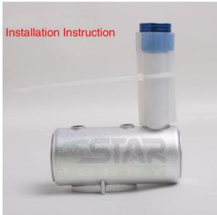
Exhaust outlet insert installed
