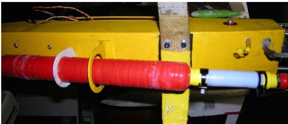
Petrol engine exhaust can wrapped with silicone rescue tape.
