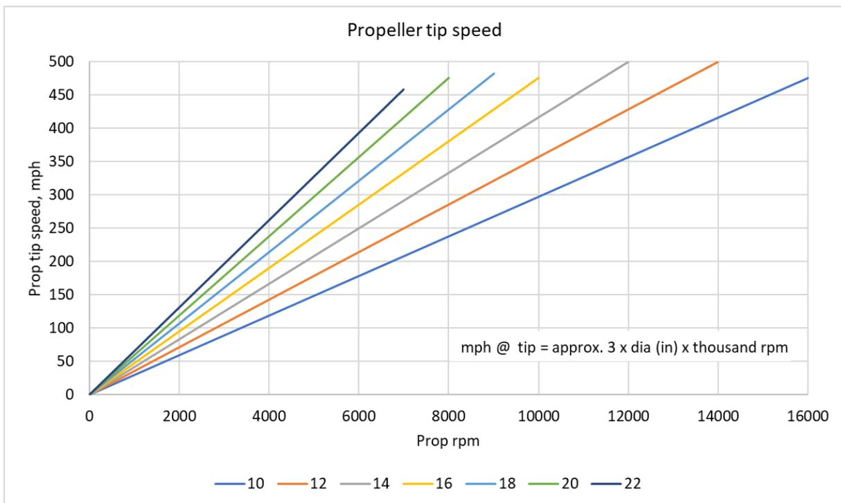
On an IC engine, the tip speed is reduced by changing the propeller pitch and/or diameter. Reducing the diameter on its own will increase the rpm, offsetting the desired reduction in tip speed. There are several permutations that are possible.
