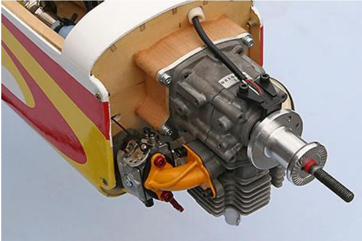
Zenoah engine with carburettor extension elbow drawing air from the fuselage to reduce induction noise
